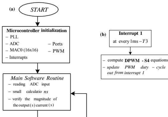
Fig. 3(a). Software control flowchart
