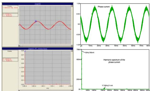
Fig. 8. – left side: waveforms and harmonic spectrum of the phase current A, obtained from oscilloscope
