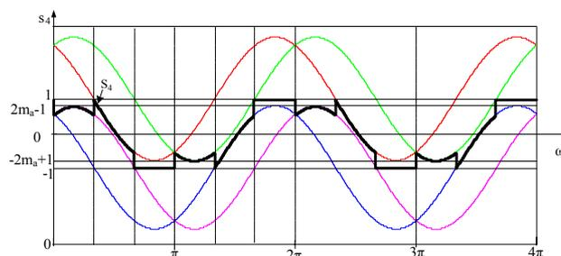
Fig. 1. The modulator signal DPWM-S4
