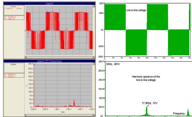
Fig. 6. – left side: waveforms and harmonic spectrum of the line to line voltage, obtained from oscilloscope
