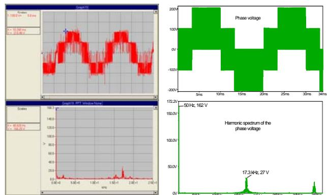
Fig. 7 – left side: waveforms and harmonic spectrum of the phase voltage A, obtained from oscilloscope.
