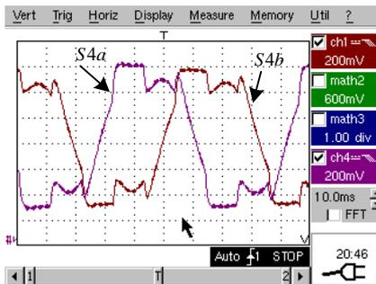
Fig. 4. Modulation signals s4a and s4b obtained by measurement
