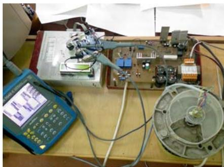
Fig. 9. Practical circuit contain: microcontroller, power three-phase inverter (made up with IRAMX16UP60A), 0,37KW motor, hall sensors for current measurements, LCD.
