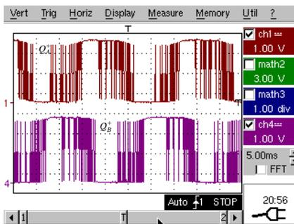
Fig. 5. Waveforms from the oscilloscope of the command signals for transistors.
