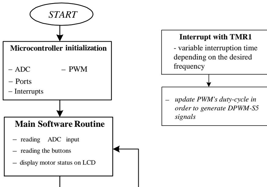
Fig. 5 – Software control diagram.
