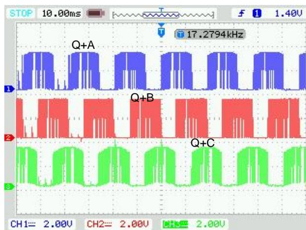
Fig. 7 – Control signals for  $Q_A^+$ ,  $Q_B^+$  and  $Q_C^+$  transistors.
