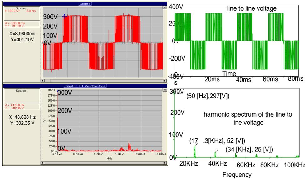
Fig. 8 – *a* – waveforms and harmonic spectrum of the line to line voltage, obtained from the oscilloscope; *b* – waveforms and harmonic spectrum of the line to line voltage, obtained by simulations.
