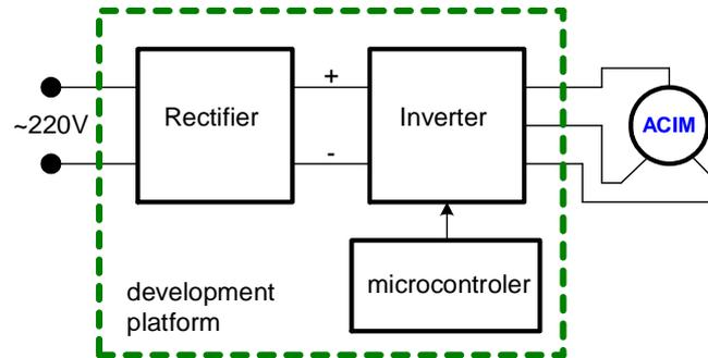
Fig. 1 – Block diagram of the development platform.
