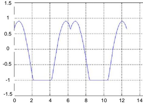
Fig. 3 – Discrete Pulse Width Modulation (DPWM) S5 signal obtained using Matlab program.
