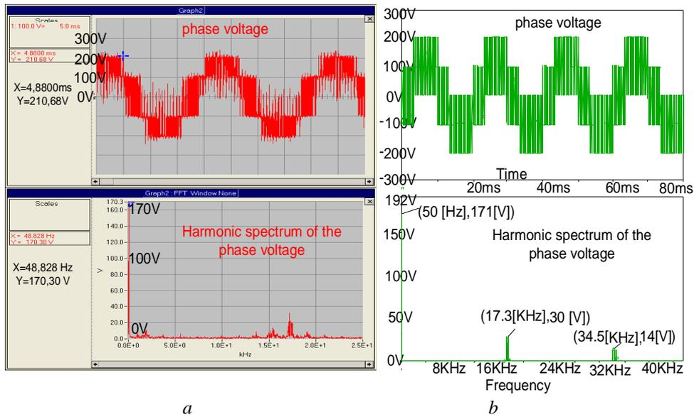
Fig. 9 – *a* – waveforms and harmonic spectrum of the phase voltage A, obtained from the oscilloscope; *b* – waveforms and harmonic spectrum of the phase voltage A, obtained by simulations.
