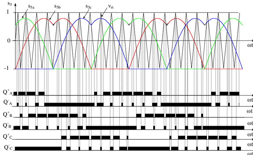
Fig. 4 – Waveforms of the reference and modulator signals and control signals for all six transistors.
