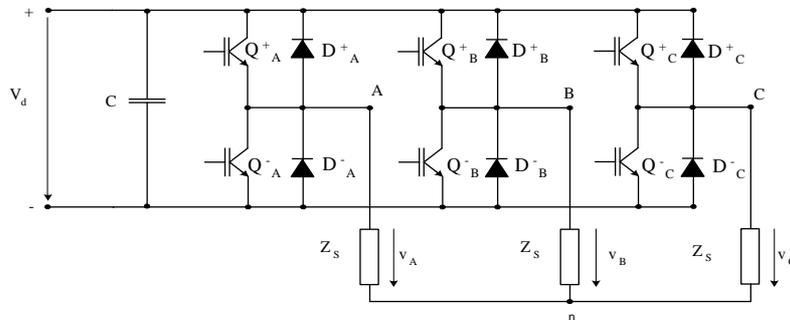
Fig. 2 – Power inverter architecture.
