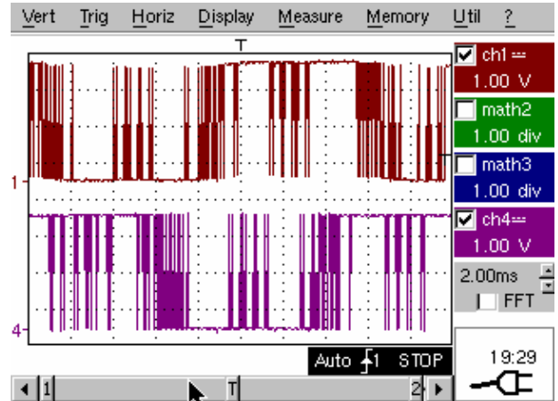
Figure 6. Waveforms from the oscilloscope of the command signals for Q_A^+ and Q_B^+ transistors.
