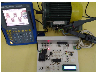
Figure 10. The practical circuit contains: three-phase inverter with microcontroller, AC machine and oscilloscope
