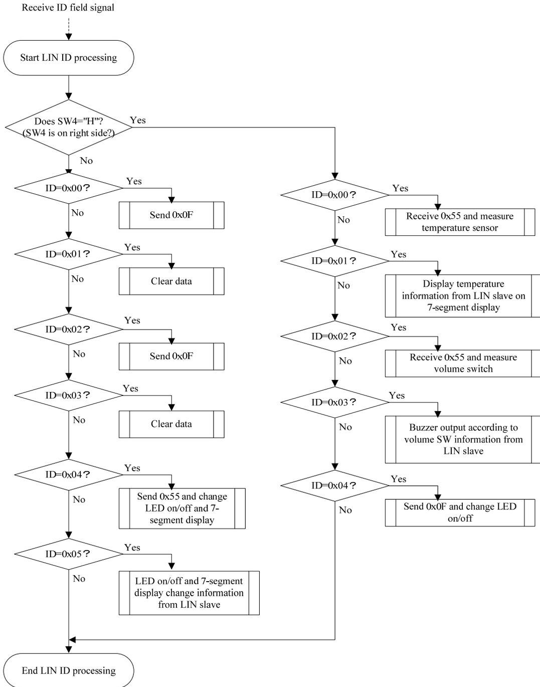
Figure 6-11 LIN communication flowchart (data processing by ID)
