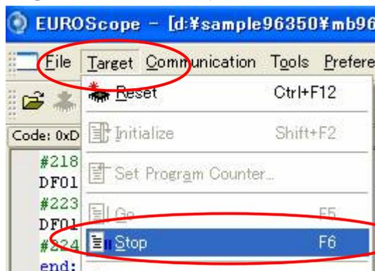
Figure 2-37 Stopping debug execution
